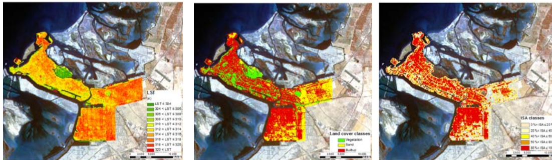
Fig. 2: example of obtained ASTER maps of LST (a, above), land cover (b, middle) and ISA percentage (c, bottom) for 10 th June 2008 image
